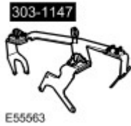
Engine lifting cradle - 4.0L 303-1147
