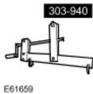
Engine lifting bracket 303-940 (LRT-12-138)
